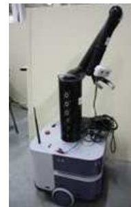
Fig 1: The robot SAM includes a 6 DOF arm and a gripper.
