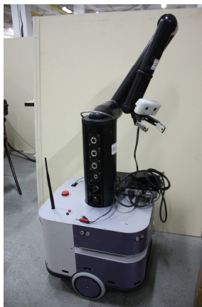
Figure 1: The mobile robot SAM, composed of a ROBULAB 10 mobile base and a MANUS arm.
